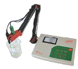
The temperature coefficient is user selectable. The pH calibration can be performed at 1, 2 or 3 points with five memorized buffers (pH 4.01, 6.86, 7.01, 9.18, 10.01). In addition, AD8000 is provided with calibration timeout alarm, GLP feature to view last calibration data and automatic HOLD feature to freeze the first stable reading on the LCD.
